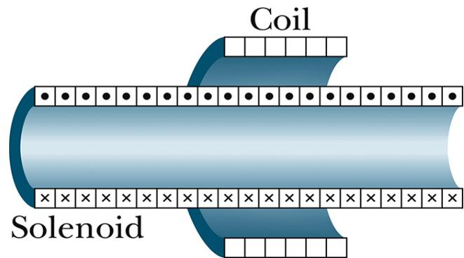
A current of  $i(t) = I_0[(3t/\tau) + (t^2/\tau^2)]$  is flowing through the solenoid, with  $I_0 = 10$  amps and  $\tau = 0.10$  sec.
