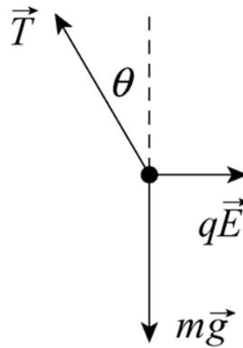
The electric field produced by the plate is normal to the plate and points to the right. Since the ball is positively charged, the electric force on it also points to the right. The tension in the thread makes the angle  $\theta (= 30^\circ)$  with the vertical.
