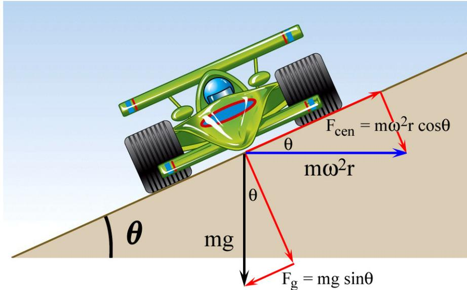
We have three forces to deal with: gravity, friction, and the so-called centrifugal force. Using the relation that  $v = (2\pi r)f = r\omega$  for circular motion, where  $\omega$  is the
