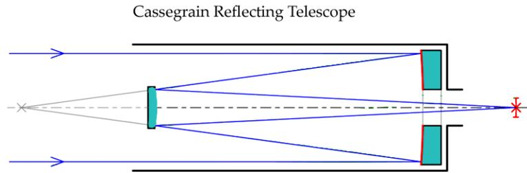
any significant effect on the image quality except to lower the light-collecting efficiency somewhat. The advantage of Cassegrain-type reflectors (there are a half-dozen variations on the basic design) is that heavy instruments can be mounted in back, along the axis of the telescope, which makes them much easier to balance and therefore to construct.
