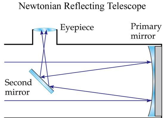
But, you say, aren't there problems with a Newtonian reflector? Won't that flat mirror in the middle of the tube block your view of the middle of the astrophysical object? Also, the flat mirror has to be held in place by wires or something. Won't an image of that superstructure (or at least a shadow of it) be superimposed on your astrophysical photography?
