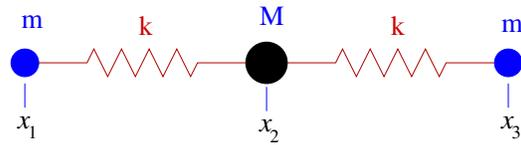
1. The linear one dimensional oscillations of a symmetrical triatomic molecule can be modeled by the configuration of a mass  $M$  connected by springs of constant force constant  $k$ , to two equal masses  $m$ , as shown. For the purposes of this model, assume that the masses are constrained to lie on a straight line. Let  $x_1$ ,  $x_2$  and  $x_3$  represent the displacements of the masses from their respective equilibrium positions.
